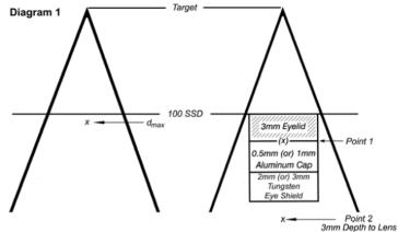
The doses are normalized to  $d_{max}$  without the eye shield (Diagram 1) using a 10 x 10 cone. When 1.00 Gy is delivered to  $d_{max}$  using 6 MeV with the shield, you get 1.08 Gy to the undersurface of the eyelid (Point 1) and 3.4% transmission to the lens (Point 2) (See table 1).
